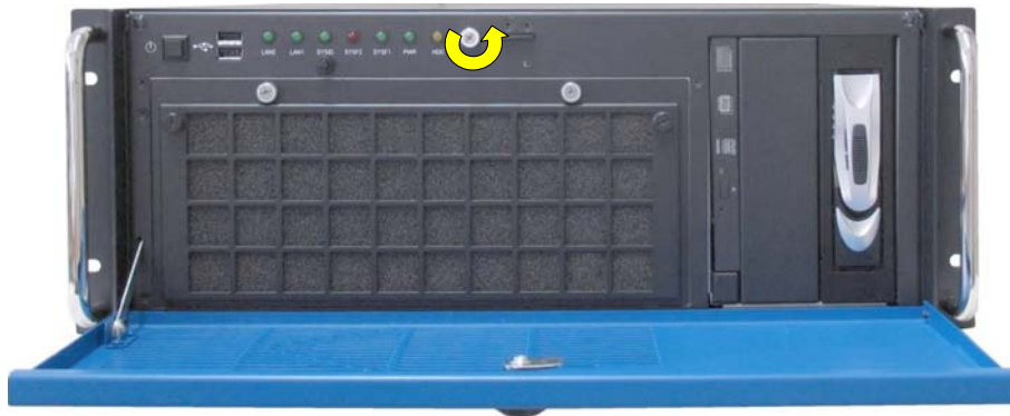
Fig. 33: Loosening the knurled cover fastening screw on the front side (shown with KTC 5520 motherboard)
