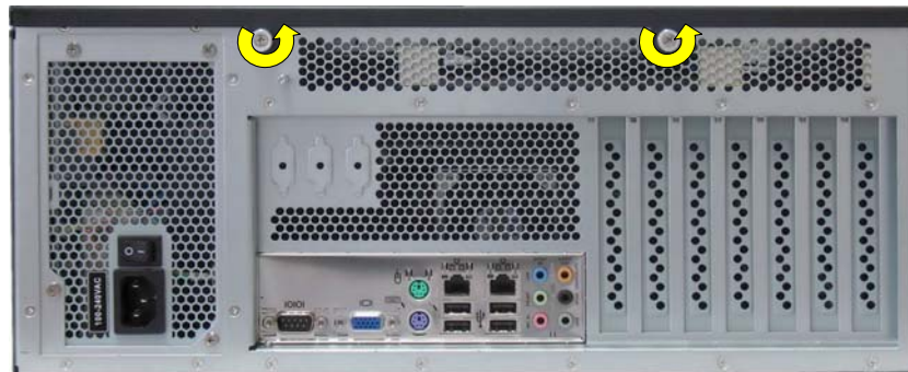
Fig. 34: Loosening the knurled screw on the rear side (shown with KTC 5520 motherboard)
