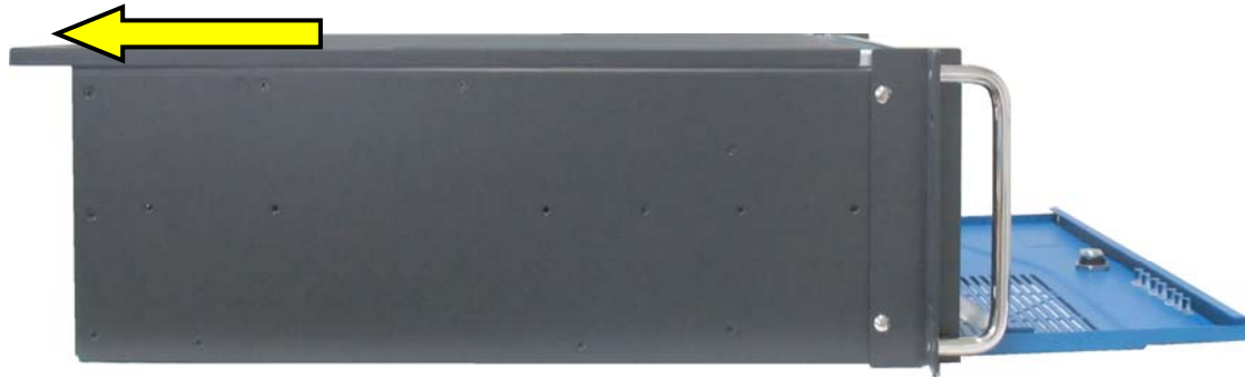
Fig. 35: Sliding back the cover will pull out the cover centering and fixing brackets from the retaining brackets of the chassis.
