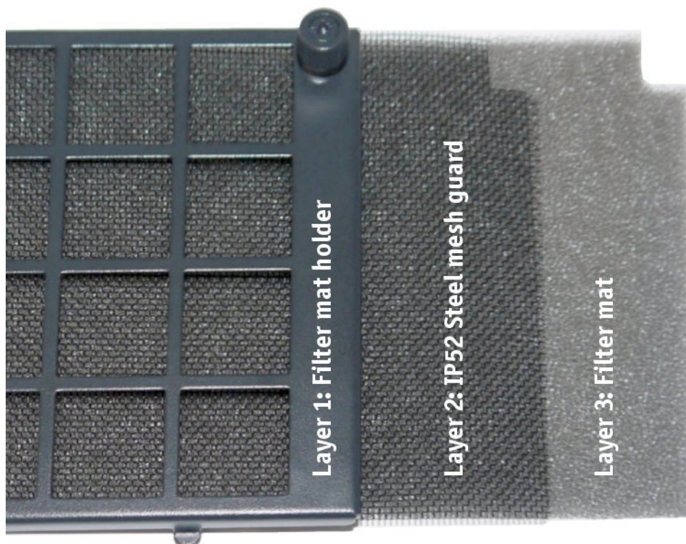
Fig. 48: Positioning of the steel mesh guard and of the filter mat in the filter mat holder (for IP52 variant only)
